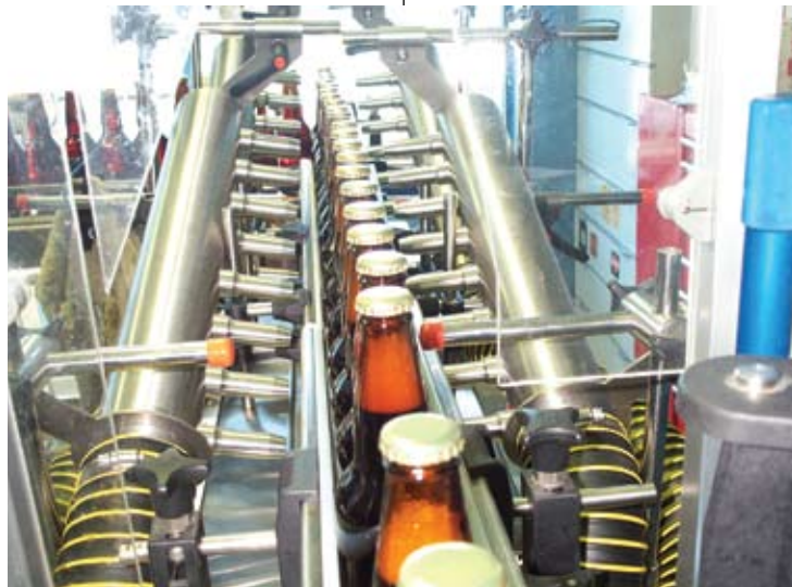
Jet Blast air knives are used to dry off bottles prior to labelling at Quebec-based beer manufacturer Les Trois Mousquetaires.
