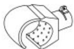
Folding reflector 72 x 70 mm push-fit on LHS 40L 107.331: Folding reflector 72 x 70 mm, push-fit
