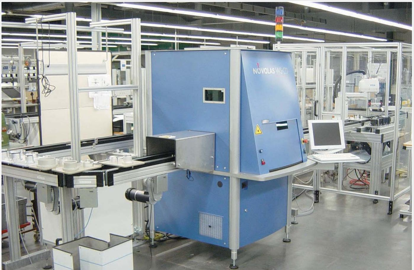
*The NOVOLAS laser systems can be optionally equipped with rotating tables or can be integrated into existing transfer systems. Many further adaptations can be implemented specific to the application.*
